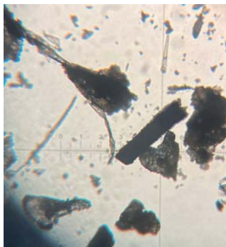
Fig. 3. Microscopy of crushed sunflower seed husk particles (ULAB XSP-137), \times 10 objective and \times 10 micrometer eyepiece, division price is 0.01 mm
