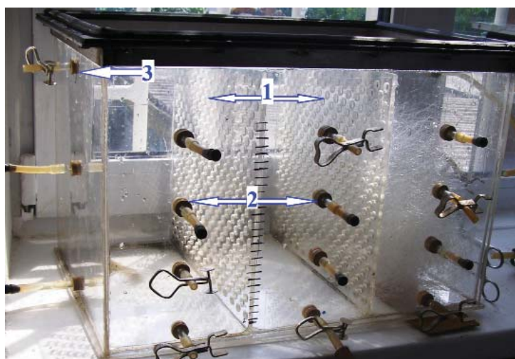
Fig. 1. The modular plexiglass installation for purification of filtrate: 1 — perforated plates for division of installation into sections; 2 — fittings for sampling of filtrate; 3 — fittings for sampling of the gas phase
