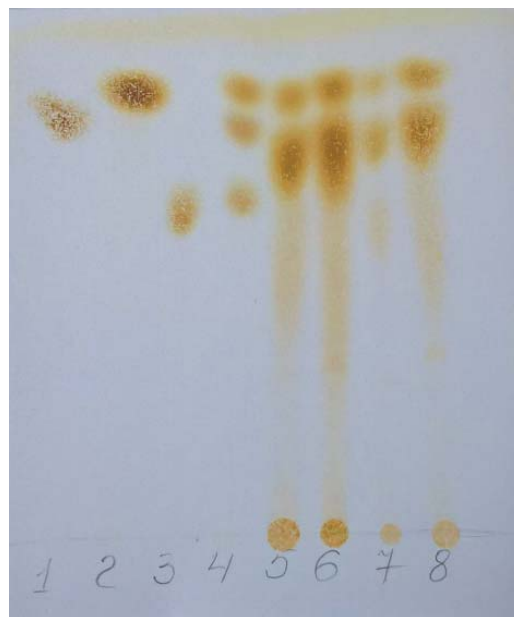
Fig. 2. Thin-layer chromatogram of RS: 1 — glucose; 2 — xylose; 3 — cellobiose; 4 — glucose+xylose+cellobiose mixture; 5 and 6 — corn cobs hydrolysates (24 and 48 h respectively); 7 and 8 — WS hydrolysates (24 and 48 h respectively)
