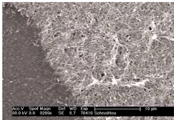
Fig. 2. SEM (FEI XL30 LaB6 SE modus 30 kV) micrograph of a MWCNT deposit.
